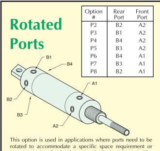
rotated to accommodate a specific space requirement or port orientation for the fittings and tube attachments. The diagram explains the options and orientation of the ports. See the specific cylinder to find availability of these options.
